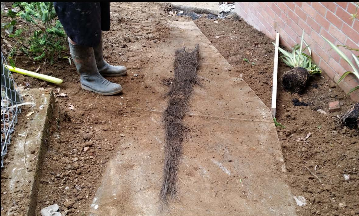
Tree Root Damage causing continual flooding to the Special Olympics Office until we got to the 'root' of the problem!
